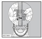
3. With a suitable spanner unscrew and remove the central rear bolt A.
